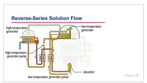
All double-effect absorption chillers are constructed from the same basic components: high-temperature generator, low-temperature generator, condenser, evaporator, absorber, two solution heat exchangers, and several pumps. There are, however, three common methods in which the solution can be circulated through the chiller: series, parallel, and reverse-series. The double-effect chiller used in the previous example employs the reverse-series flow cycle.
